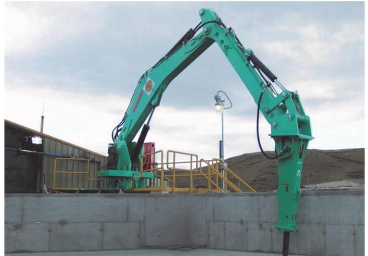
**Proper Set-Up:** The key to long equipment life and top production is to start with the boom placed in exactly the right spot. When working in your target area, a boom is positioned in its "sweet spot" when it is arched symmetrically and the cylinders are in their mid-positions. Tramac engineers will gladly work with you to find the right boom base position so you can reach the areas of top priority.
