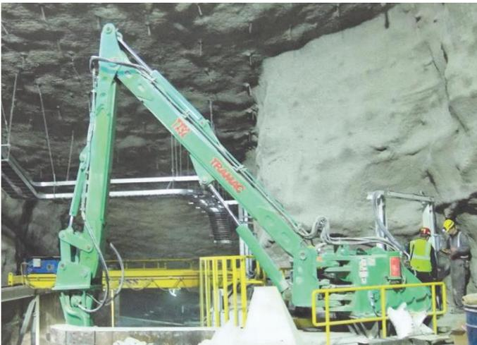
*Tramac's TX Series Rock Breaker Boom Systems are Extra Heavy-Duty assemblies for large breakers at demanding, high-production work locations. These designs are the beneficiaries of many years' experience in providing rock breaking equipment to demanding mineral mines and crushed stone producers worldwide.*
