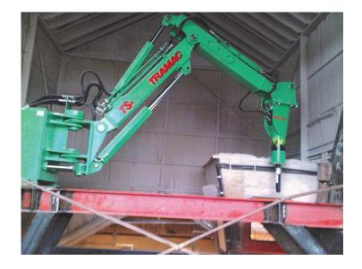
Increased Safety & Production: Increase safety around your primary. Eliminate the need for a worker to enter the area. Increase your up-time. Provide a steady flow of materials. Break rock, pull, poke, and stir material. Reach back into the hopper, work down along the feeder area, and into the crusher with smooth precision of control.
