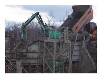
Tramac's TSH Series Rock Breaker Boom Systems provide unmatched reliability when the job calls for breaking light to medium hard rock with breakers up to 3,000 ft. lbs. These designs offer overall value, are heavy-duty constructed and relatively light in weight for easy installation.
