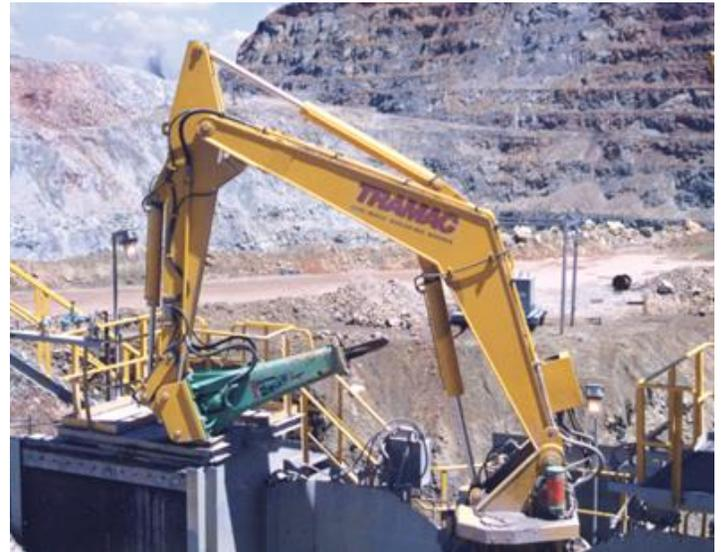
**Auto Lubrication:** Auto lube systems are frequently specified. They include the breaker and all boom lube points. Standard with TR systems is a manually fed lube system that brings the lines serving all points to two bulkhead locations.
