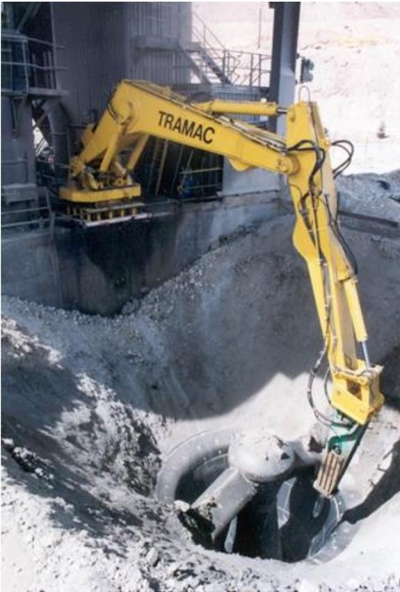
*Tramac's TR Series Rock Breaker Boom Systems are designed for high performance, increased safety, and long life when mounted over large capacity crushers. These designs are beneficiaries of many years' experience working in large crushers around the world. Tramac's users list includes some of the most prestigious names in Mines and Mining Engineering Firms.*
