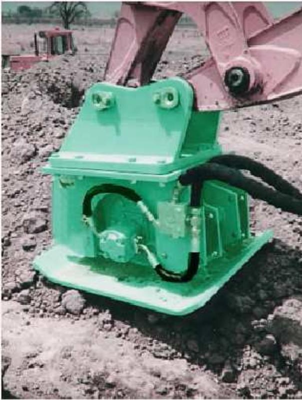
Muscle Mate compactor's operating system combines maximum eccentric weight with precise proportions of amplitude and vibration frequency that will generate the most productive centrifugal force. They are capable of handling the toughest compaction jobs, and are available in sizes to fit carriers from 3,000 up to 100,000 lbs.
