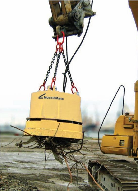
***The self-contained hydraulic magnet for cleaning and separating iron and steel from waste concrete and debris is ideal for demolition and recycling!***
