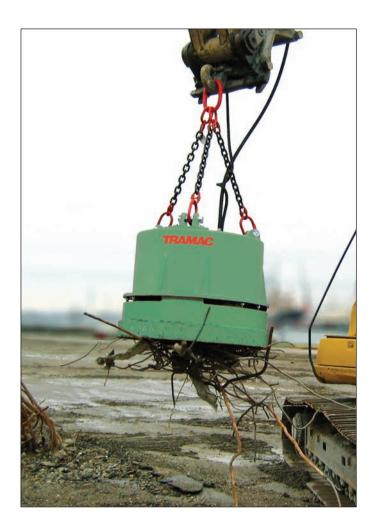
The new self-contained hydraulic magnet for cleaning and separating iron and steel from waste concrete and debris is ideal for demolition and recycling!
