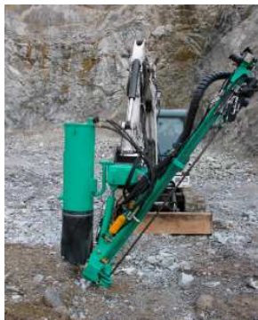
Large coverage due to the excavator boom and the +/- 45° swing cylinder on CPA
