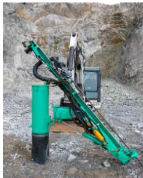
Large coverage due to the excavator boom and the +/- 45° swing cylinder on CPA
