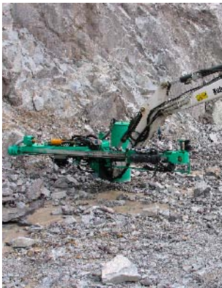
Large coverage due to the excavator boom and the +/- 45° swing cylinder on CPA
